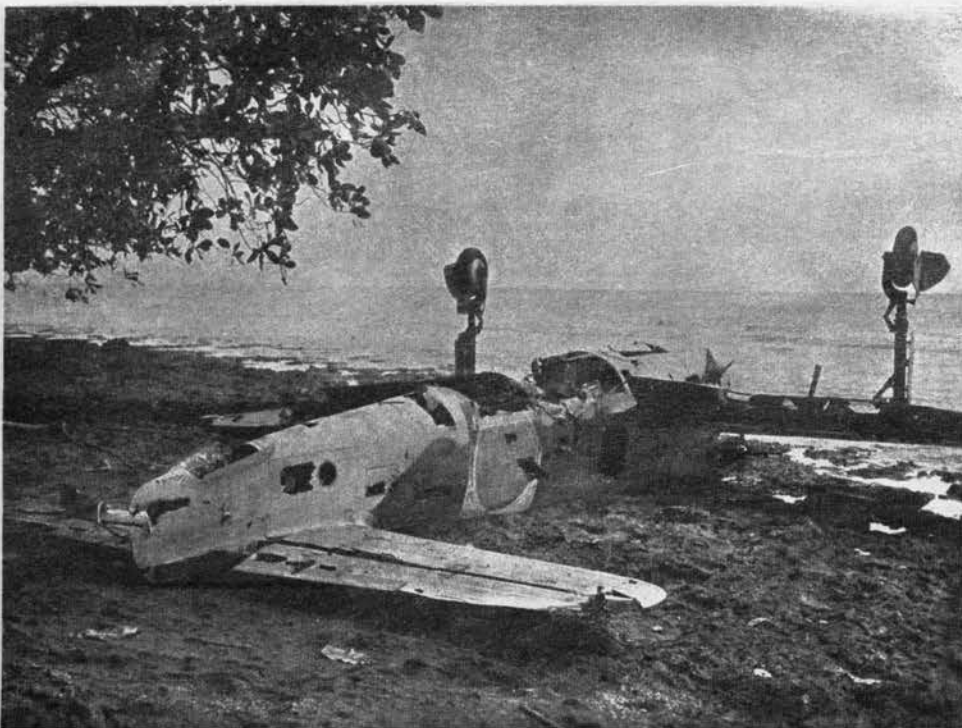
Wrecked Judy supplied early technical intelligence on new type. Note the distinctive features: deep flat-sided fuselage, bladelike projection at tail, high-set tailplane, midwing.
